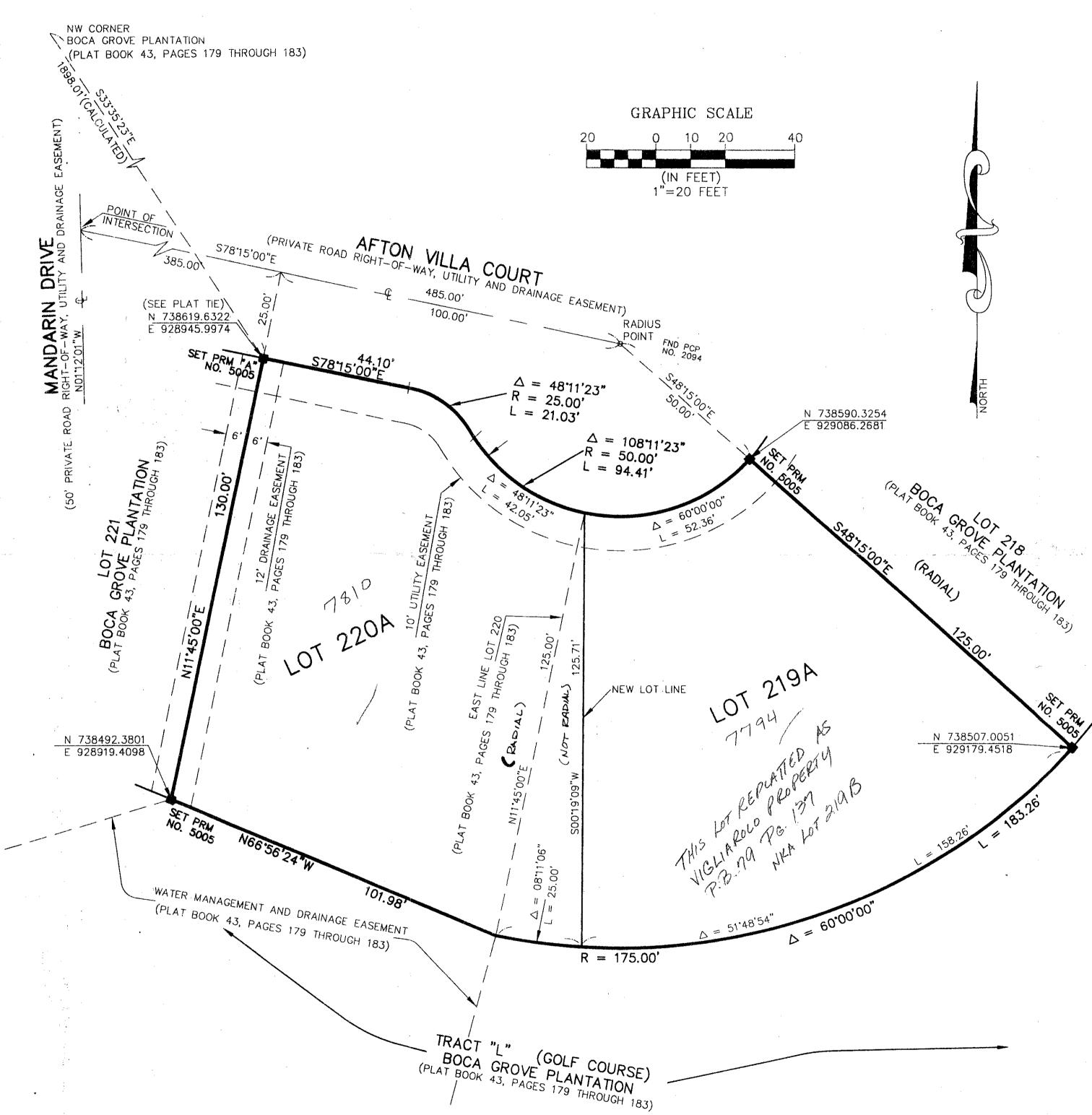
NOTES COORDINATES, BEARINGS AND DISTANCES COORDINATES SHOWN ARE GRID DATUM = NAD 83 1990 ADJUSTMENT ZONE = FLORIDA EAST LINEAR UNIT = US SURVEY FEET COORDINATE SYSTEM 1983 STATE PLANE TRANSVERSE MERCATOR PROJECTION ALL DISTANCES ARE GROUND SCALE FACTOR = 1.0000265GROUND DISTANCE X SCALE FACTOR = GRID DISTANCE (CLOCKWISE) N11'45'00"E(PLAT BEARING) BEARING ROTATION N11'48'05"E(GRID BEARING) (PLAT TO GRID)
